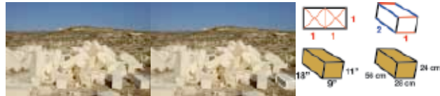
Figure 12: Measured dimensions of modular blocks and the ratio which appears in the block.
