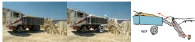
Figure 11: Running band which loads the dressed blocks onto the means of transport.
