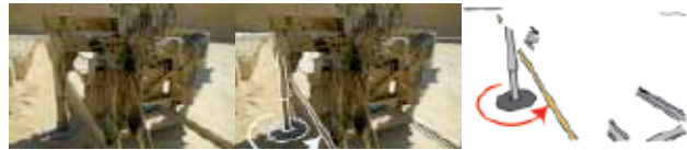
Figure 9: The saw for horizontal cutting of stone is used when the stone has already been cut vertically.
